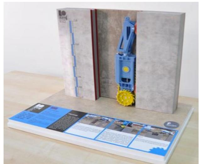
A 1:20 3D scale model was on display showing the shape of the trimmer and the construction stages that make up the TTMJ system.
