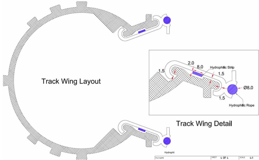
*Fig. 8 - Arrangement of the water stop slipped over the track wings*
