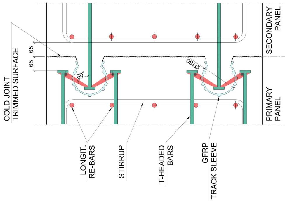
*Fig. 7 - Arrangement of the headed bars for the Tension Track*
