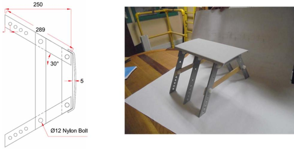
Fig. 4 - Prototype of the GFRP cage spacer
