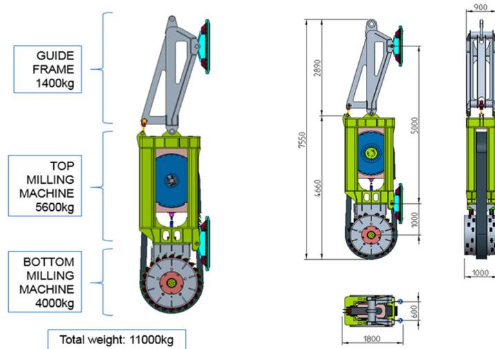
Fig. 5 - TTMJ machine dimensions and weight
