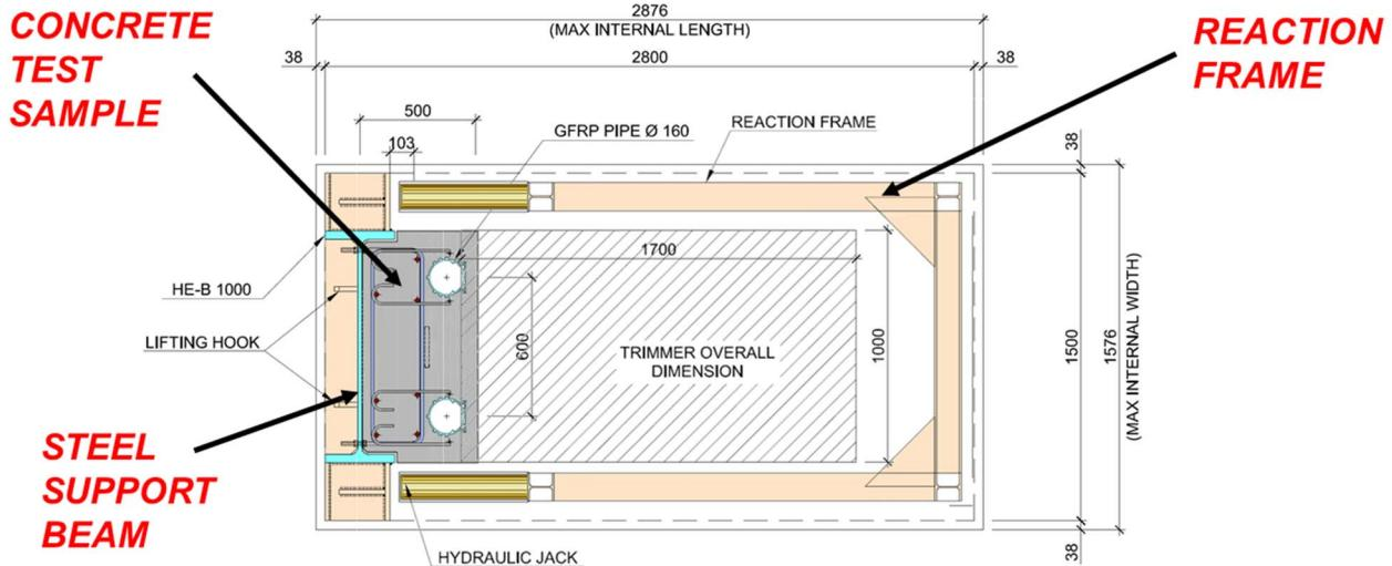
Fig. 14 - Test concrete beams – reaction frame
