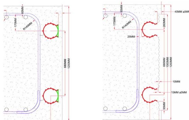
Fig. 3 - Track Cast into Panel (left) and Panel joint after trimming (right)
