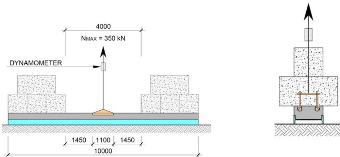
Fig. 15 - Pulling test
