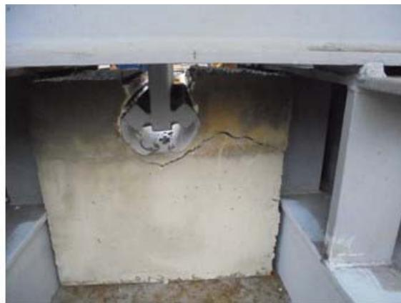
Fig. 10 - Samples of track pull out tests
