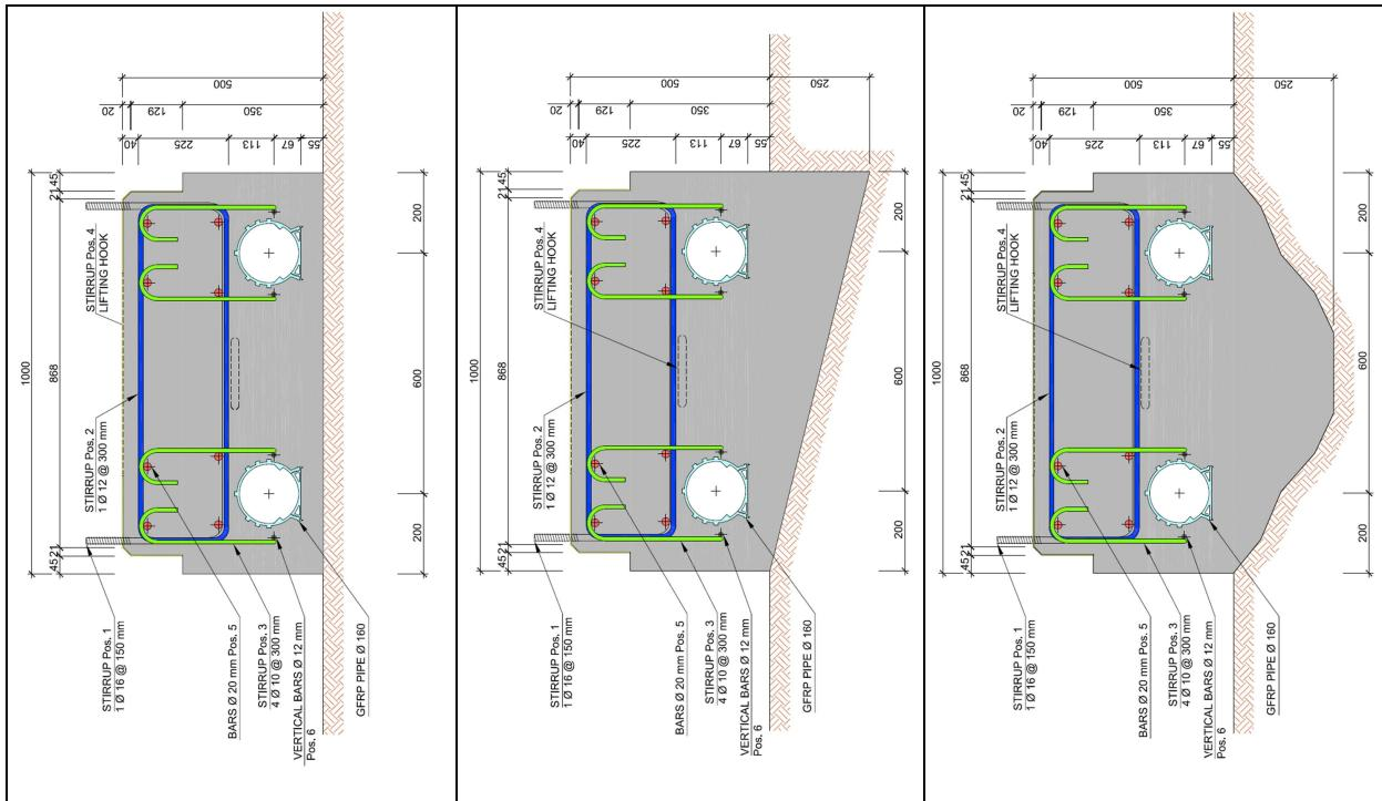
Fig. 13 - Test concrete beams - Flat face type (left), slanted face (center) and bulged (right)
