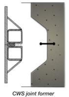
However, a joint formed by over-cutting the concrete with the mill cannot accommodate a water stop and the shear connection between the panels is limited.
